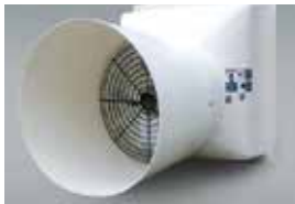
Made of durable fiberglass, AP's optional discharge cones boost fan output by as much as 15%. The 14"-36" fiberglass cones are provided as a one-piece unit and 50" & 54" in an easy to ship and assemble 3 or 4-piece units.
