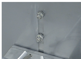
The ML Series feeding shelf can be raised or lowered using a manual 3-position bolt pattern.
