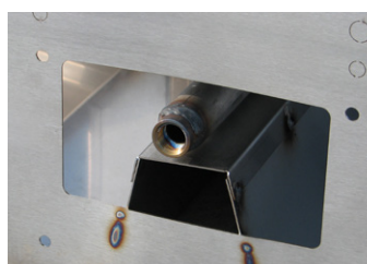
STEEL WATER LINE CONNECTION
