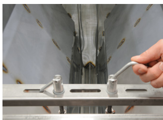
A simple hand crank adjusts the feed gate on the Standard wet/dry feeder.
