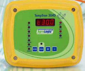
The first stage has a minimum ventilation on/off timer and an on/off timer for the cooling that can be set by the user.
